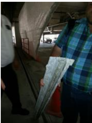
Expansion joint from the East garage that was removed
